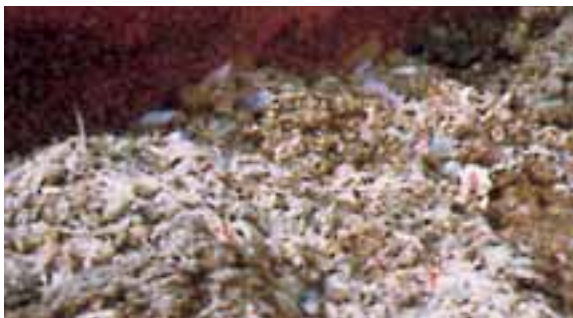
Screenings in a container
